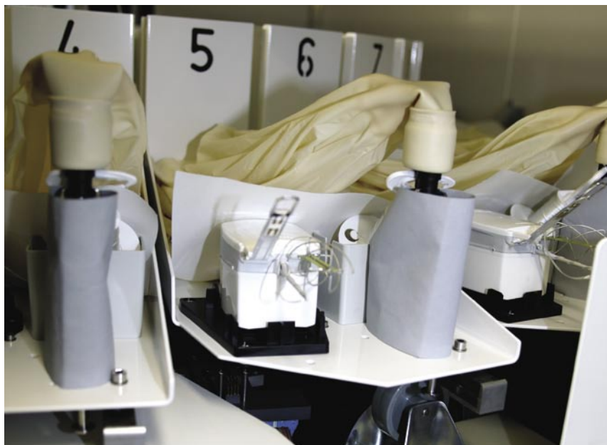
An attendant only needs to reload the daisywheel with radiosondes and balloons every 12 days.
